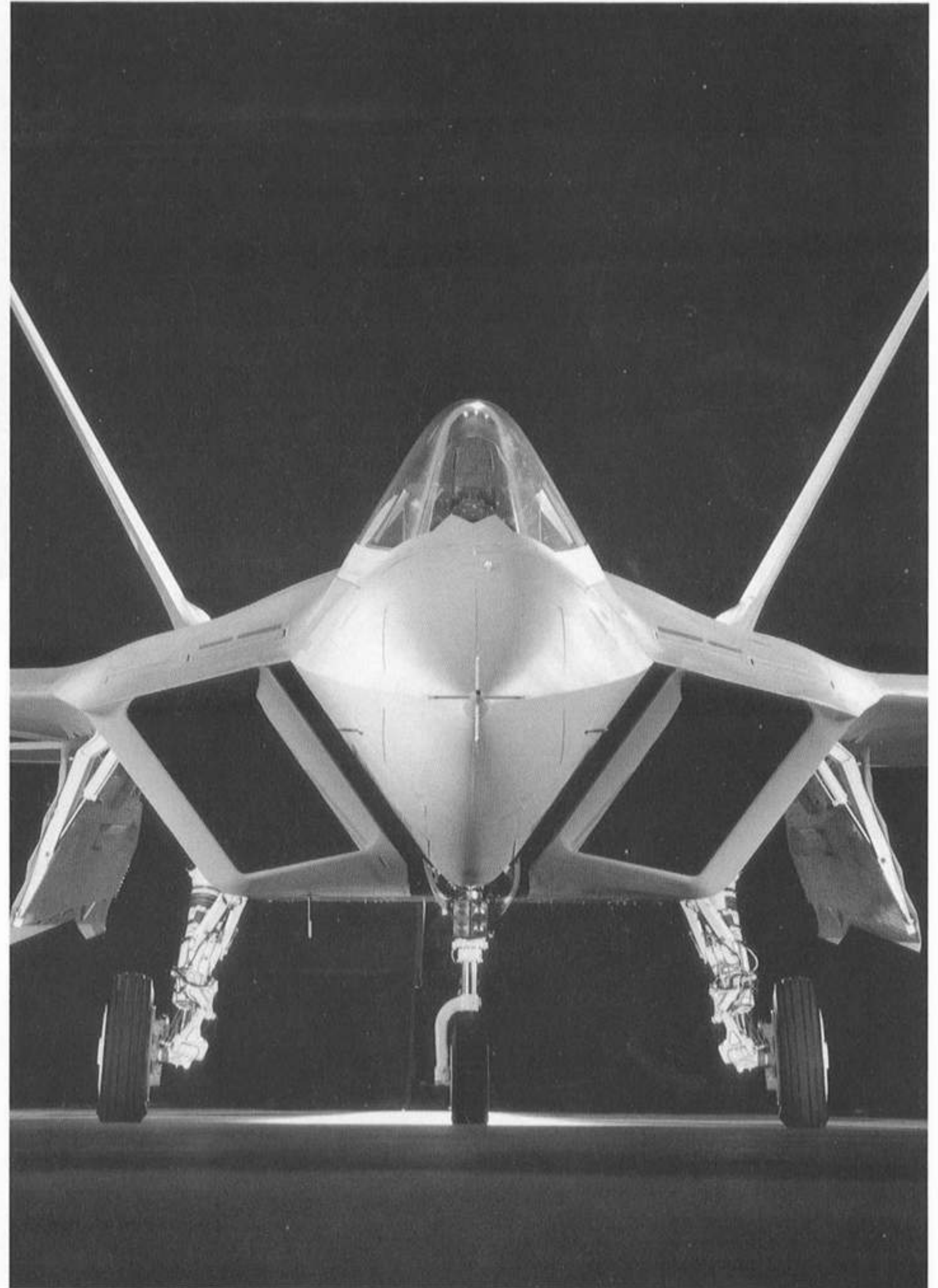
The YF-22A's cockpit canopy has low observable shape to avoid radar reflection. Also the canopy should have the radar absorptive coating, but this is lacking on the prototype.
