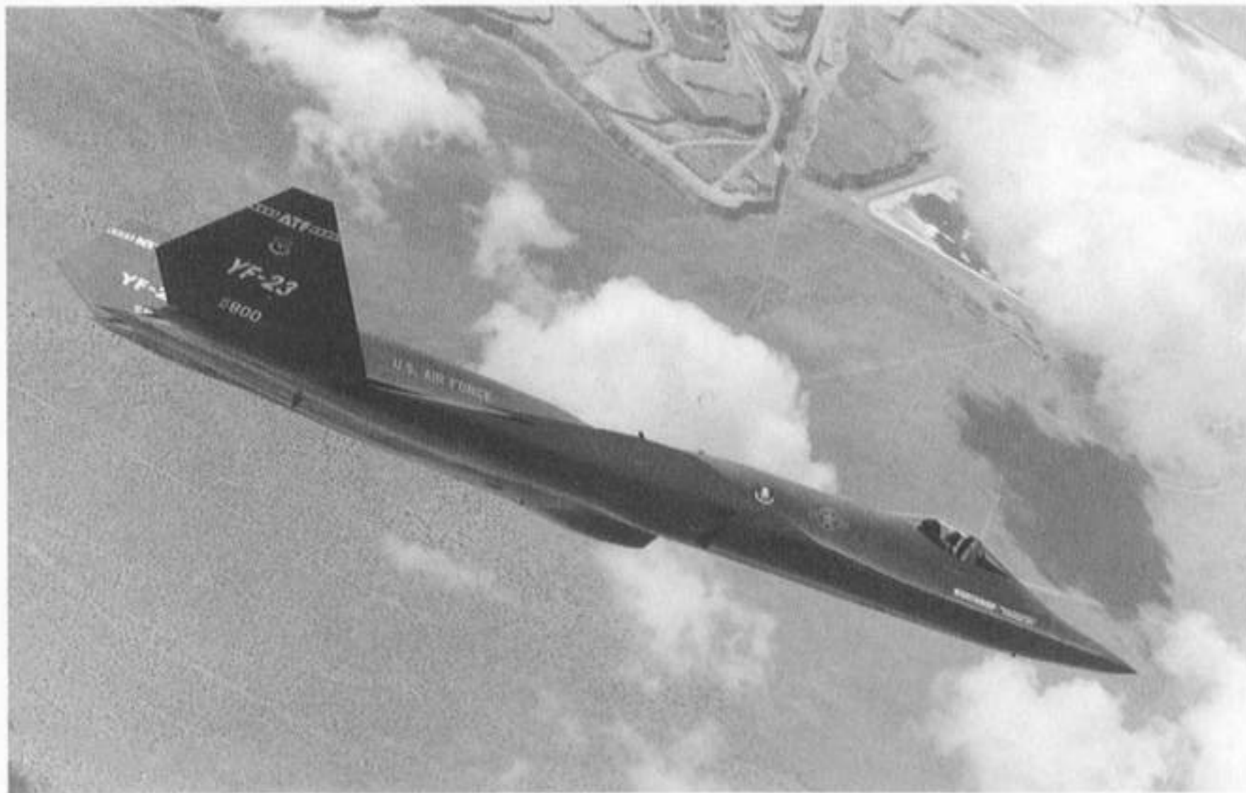
The YF-23A ATF's nose to wing chine runs horizontally along both sides of the cockpit to join at each wing root. The chine design balances low observable and aerodynamics characteristics.
