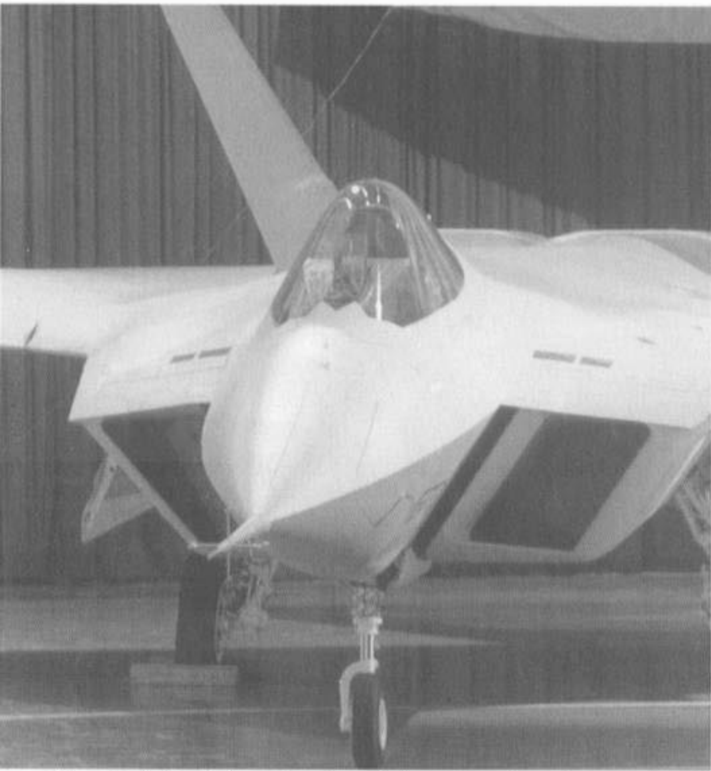
The avionics bay is located in front of the engine inlet and the radome is in the mid-nose section, all have serrated outlines to reduce radar reflection.
