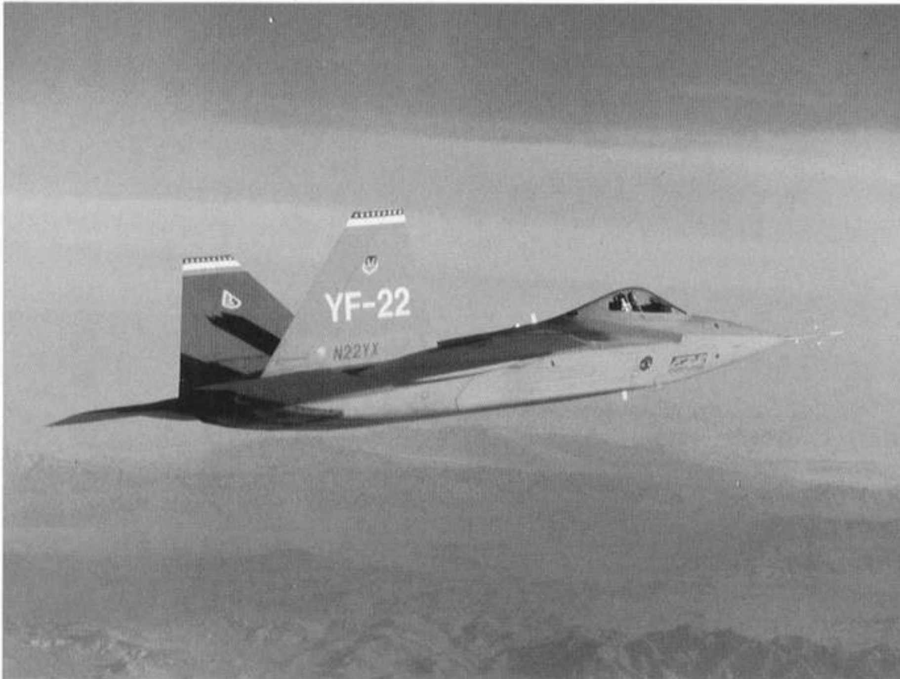
The YF-22A features new designs that has increased its survivability and combat capability. This is made possible by the use of stealth technologies and advance sensors to reduce threat reaction time, nullify enemy fighter radars for the first-look, first-launch, first-kill capabilities.
