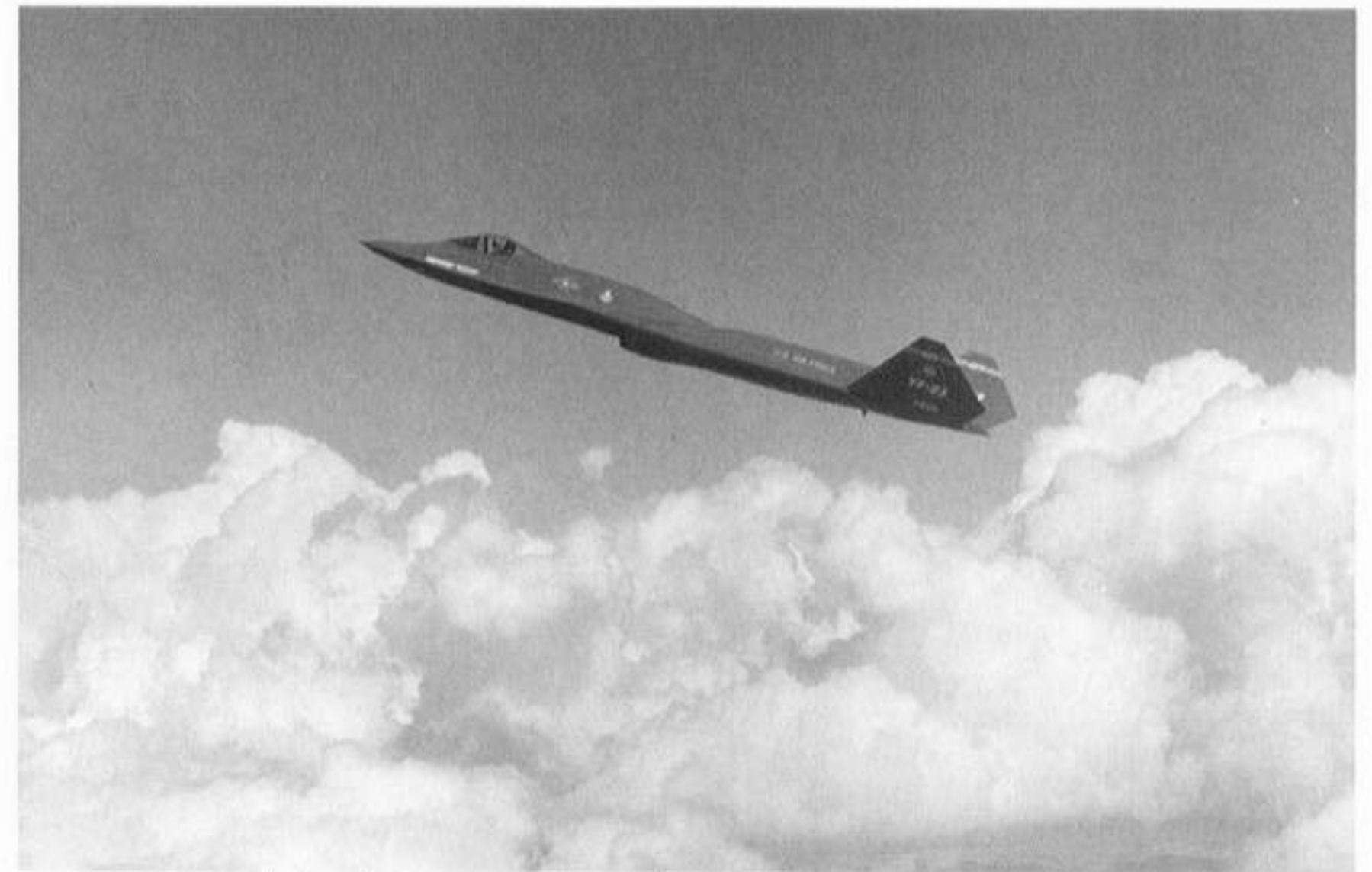
Supersonic flight of the YF-23A was achieved on September 18, 1990 without using afterburner. One of the main goals of the ATF is to be able to sustain supersonic cruise without using afterburners, the "Supercruise" performance.
