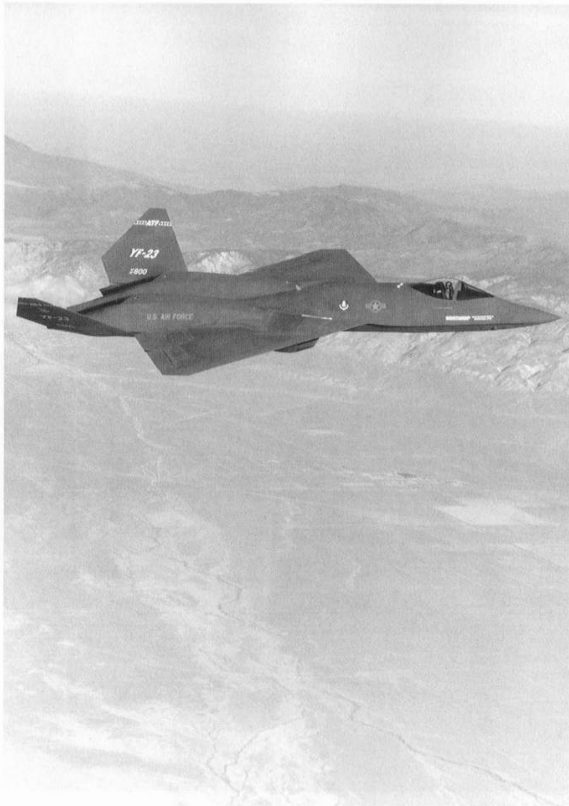
During the flight evaluation tests, the YF-23A has reached a maximum altitude of 50,000 feet and a maximum speed of Mach 1.8 using afterburner.
