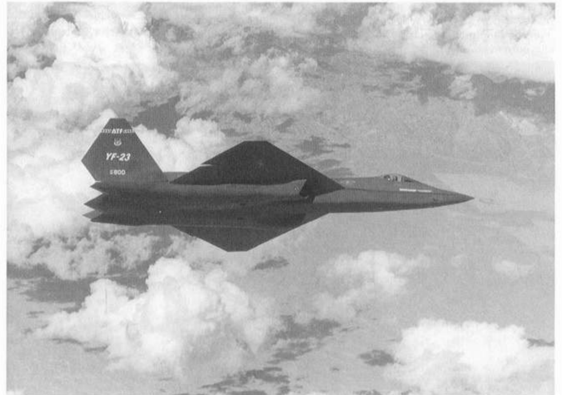
During the flight evaluation tests, the YF-23A has reached a maximum altitude of 50,000 feet and a maximum speed of Mach 1.8 using afterburner.
