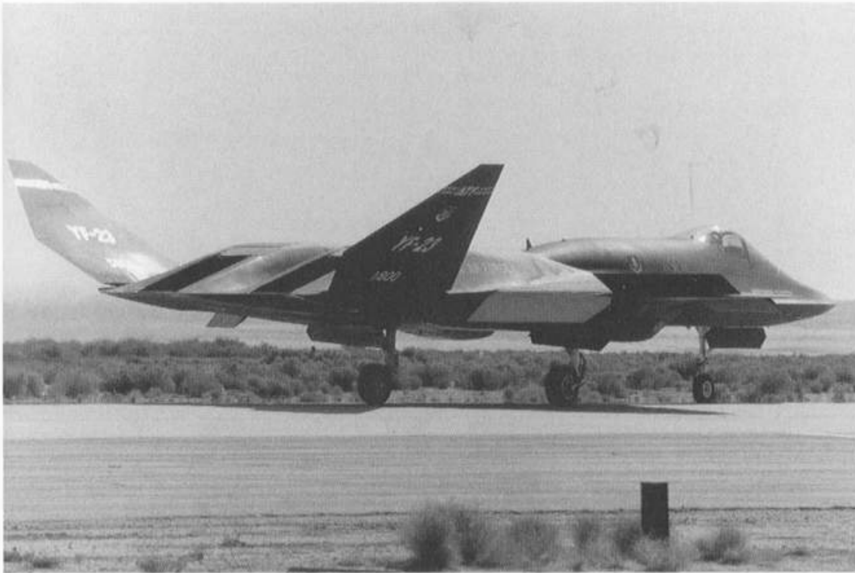
The YF-23A ATF demonstrator was unveiled on June 22, 1990 at Edwards Air Force Base, California. The futuristic looking twin-engine plane blends low-observable and aerodynamic technologies into a complex, but balanced design. The YF-23A has more emphasis on stealth than its rival, the YF-22A, which looks more like an air superiority fighter.
