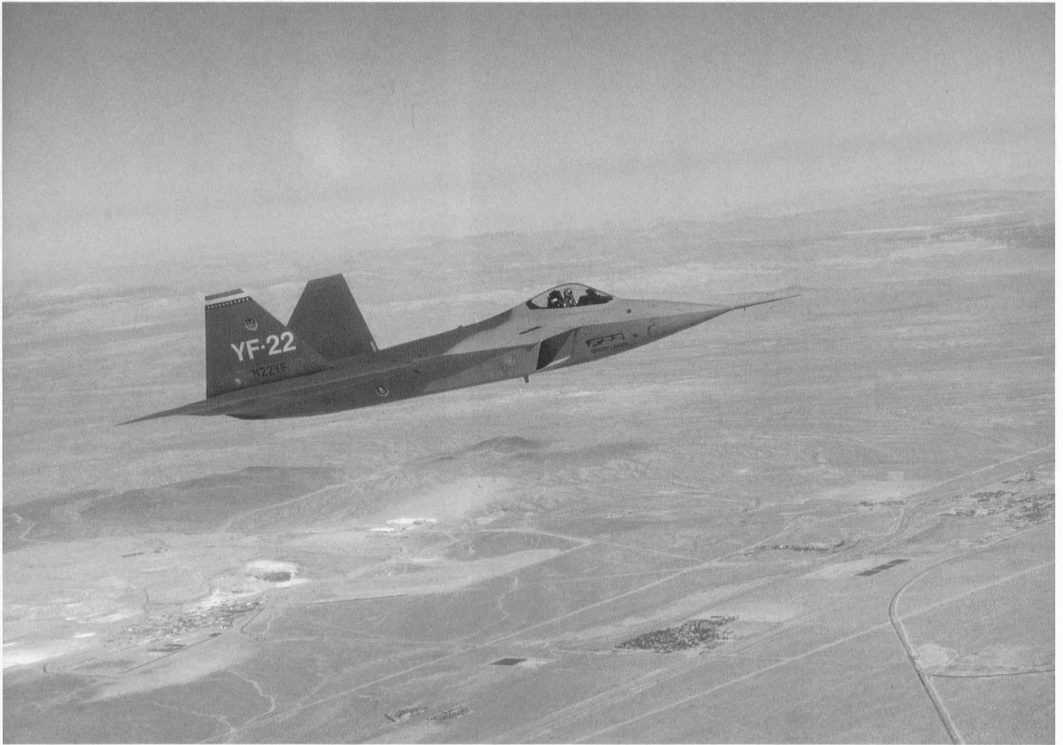
Due to its supercruise capability, the YF-22A has a 25% increase over the F-15 and a 35% increase over the F-14D in combat range.
