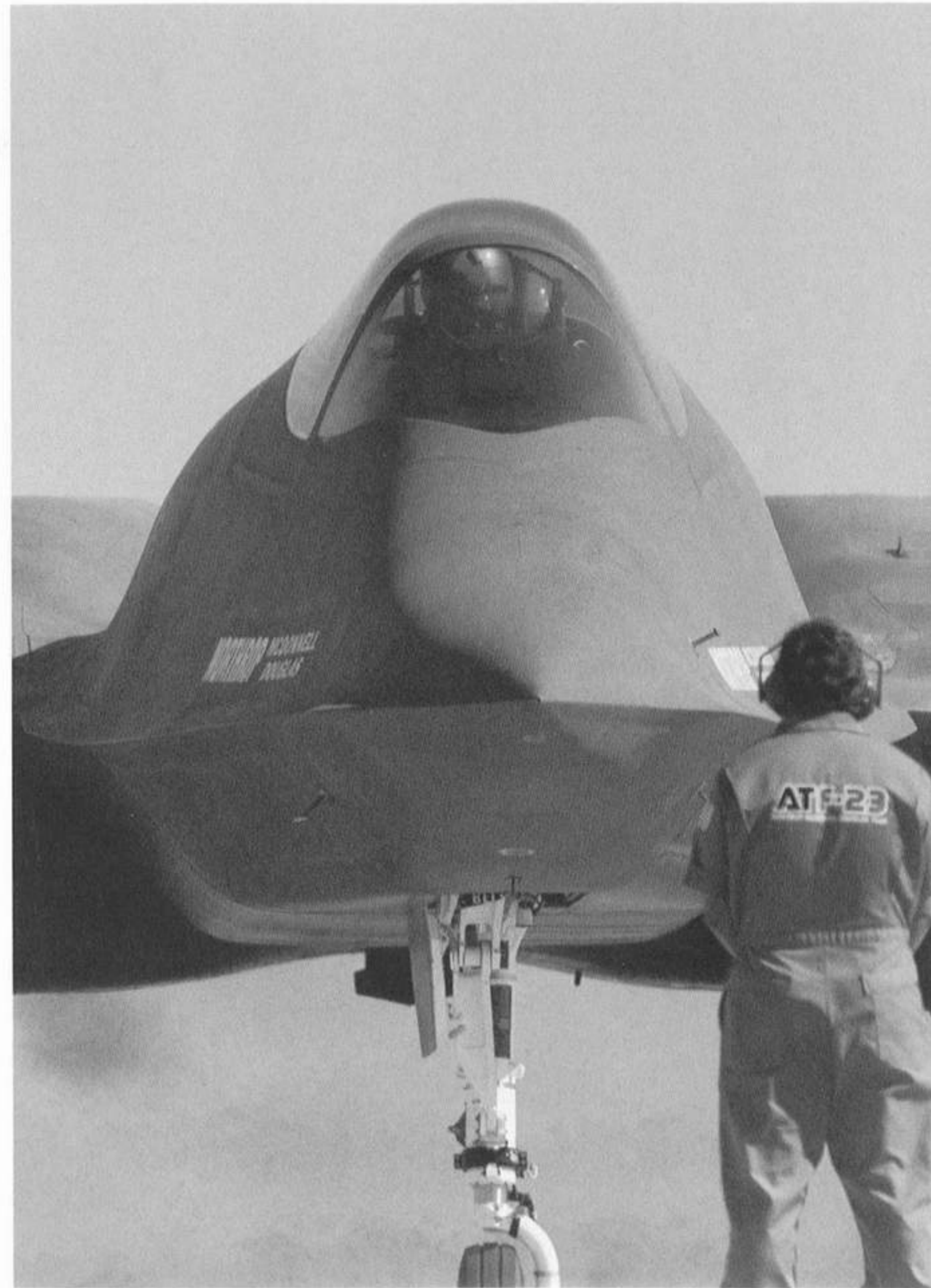
The YF-23A has chines that bear resemblance to the Lockheed's SR-71 Blackbird, presumably for added stability at high speed. The small nose section implies a smaller scanner is in place.
