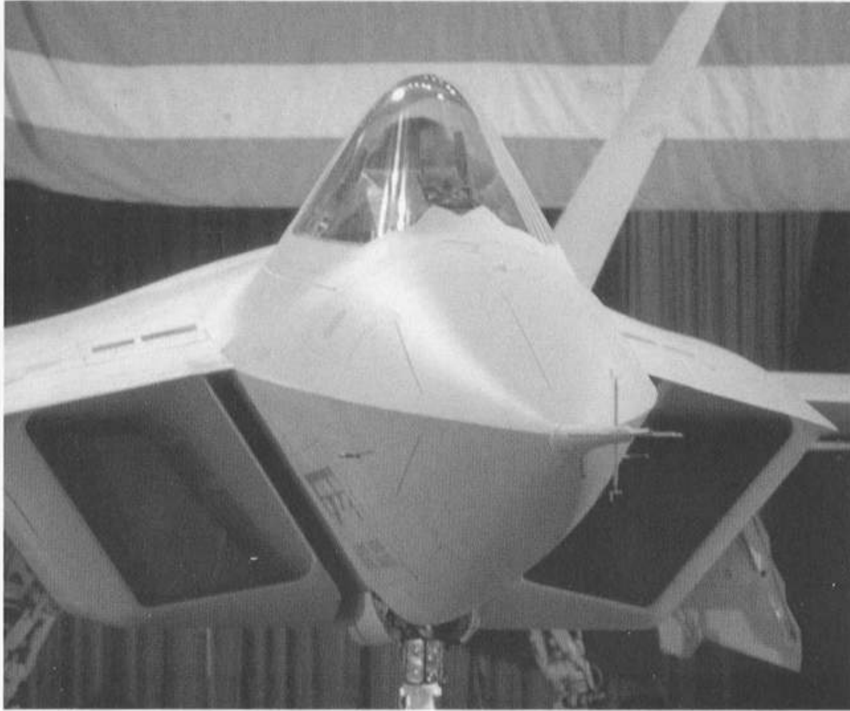
The YF-22A's cockpit canopy has low observable shape to avoid radar reflection. Also the canopy should have the radar absorptive coating, but this is lacking on the prototype.
