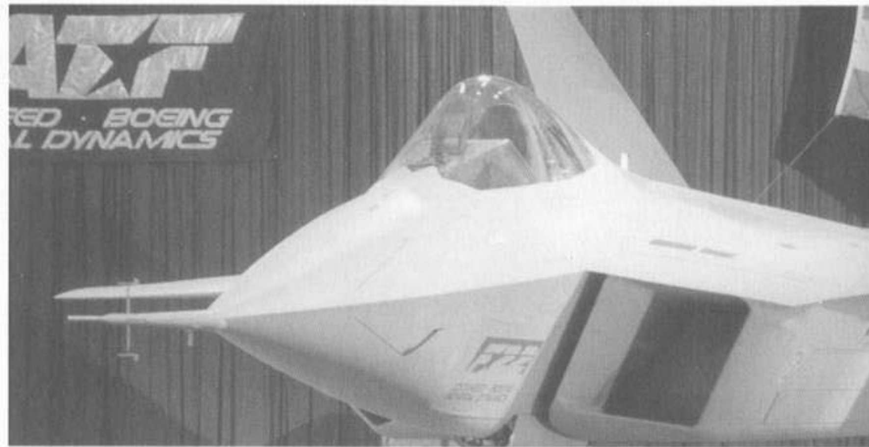
The YF-22A is more angular in design than the YF-23A, reflecting the Lockheed experience with the F-117A. It appears more compact too, but is only 3.2 feet shorter in length. The YF-22A has length of 64.2 feet and wingspan of 43 feet.
