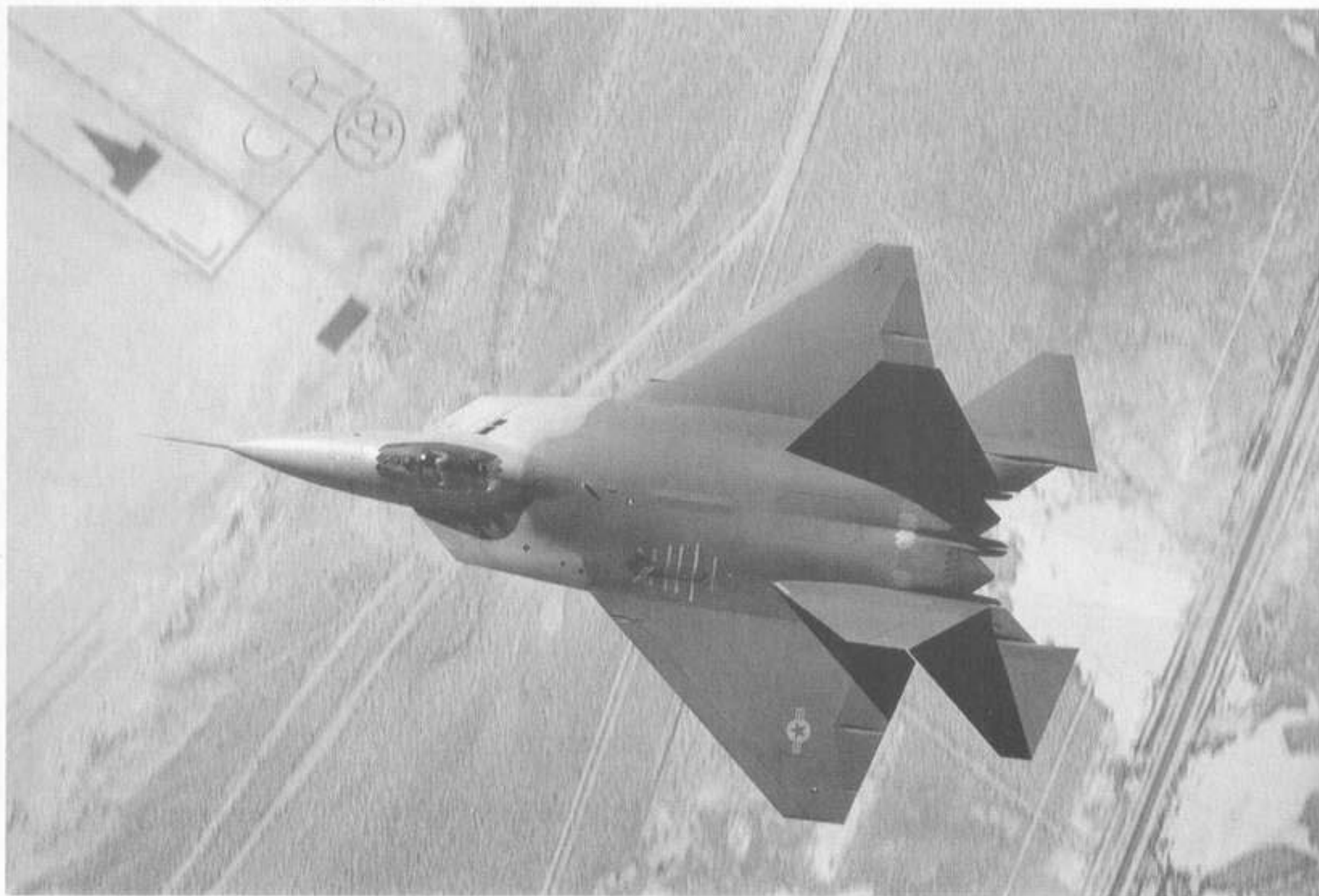
The YF-22A has a subtle chine joining the upper and lower nose halves in a sharp line. The flow control panels, two on top of each inlet, marked "NO STEP" is for control of airflow on top of the wing.
