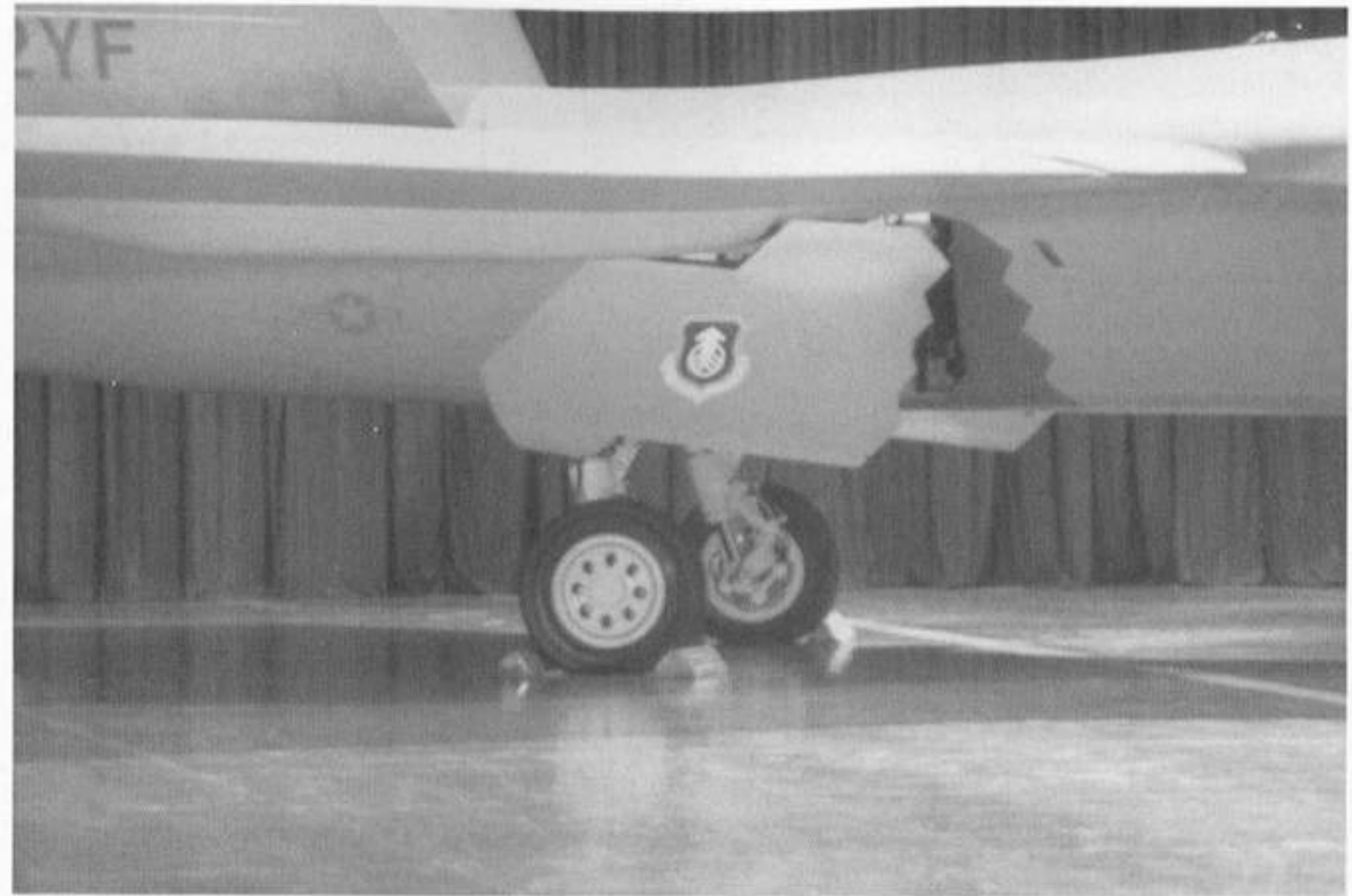
Most openings such as radome, missile doors, canopy, avionics bay and landing gear doors have serrated edges to reduce radar reflection. The YF-22A is built with radar-adsorbing materials.
